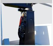
Ground level emergency lowering from the chassis (pedestal mounted valve bank)
